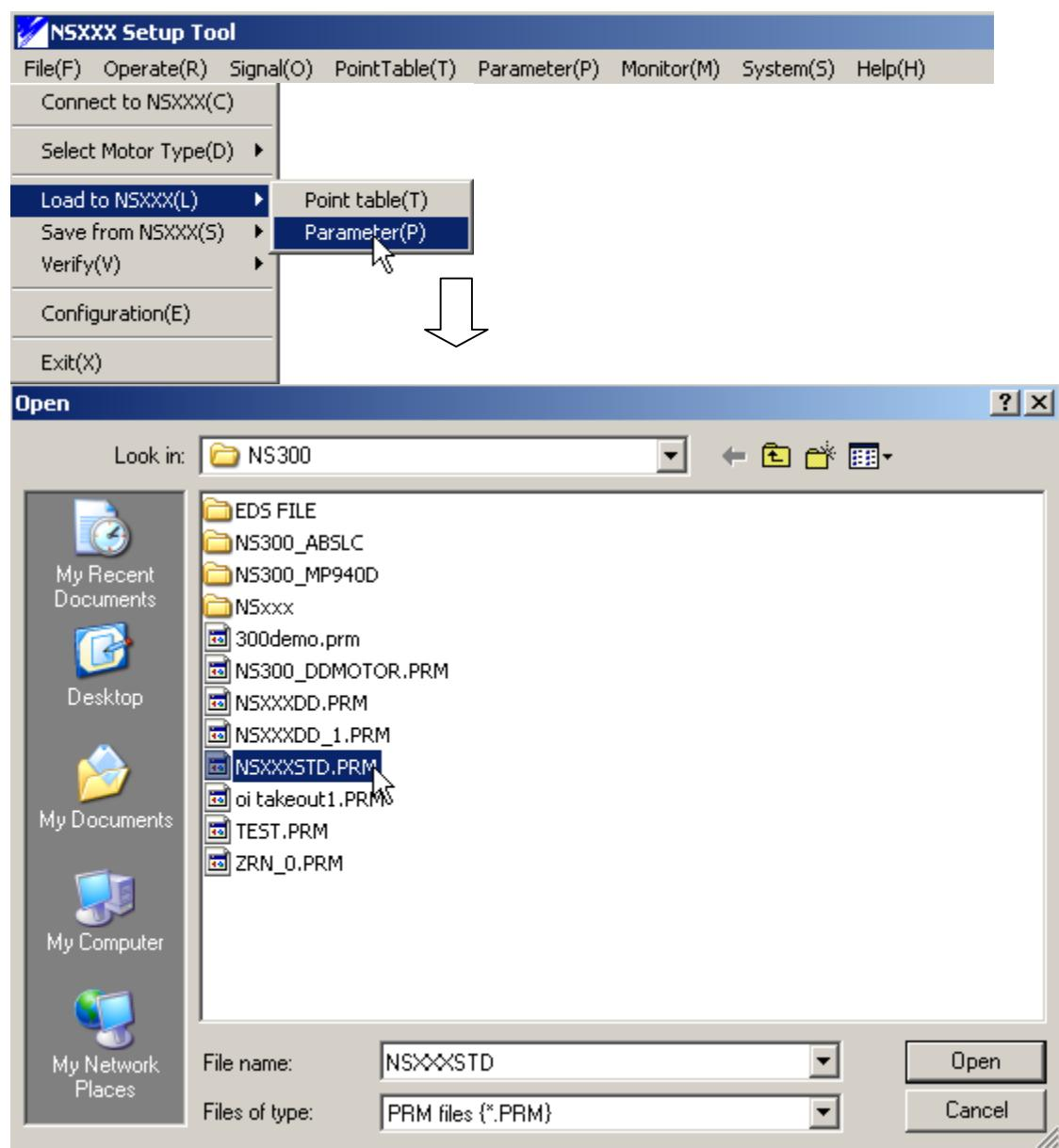
After editing any parameters or loading new parameters, carry out a system reset to save the parameters to non-volatile memory. Choose Reset module (M) from the System (S) Menu.
