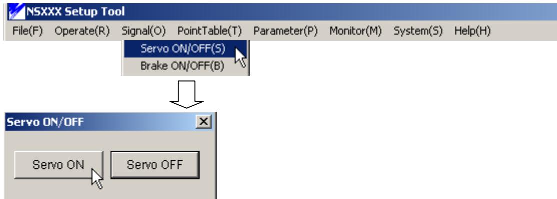
The SGDH display should read, “run”. If it reads “bb”, check that the EMG STOP circuit is wired correctly and has not disabled the drive, or disable the EMG STOP input by setting Pn081B to 0000.
