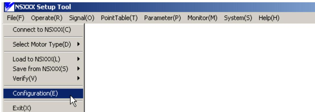
We assume that the set up is for mm. Change the display unit from "None" to "mm". Change the command unit from 0.01 to 0.001.
