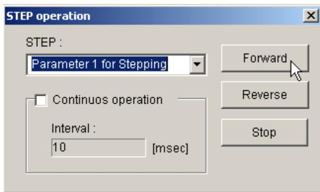
Select Forward or Reverse button. Do not select continuous operation while demonstrating the STEP operation. The motor should index to the stored value at the feed speed for positioning parameter Pn821. If there is no motion, then check that the servo is enabled, EMG STOP input, P-OT input and N-OT input.
