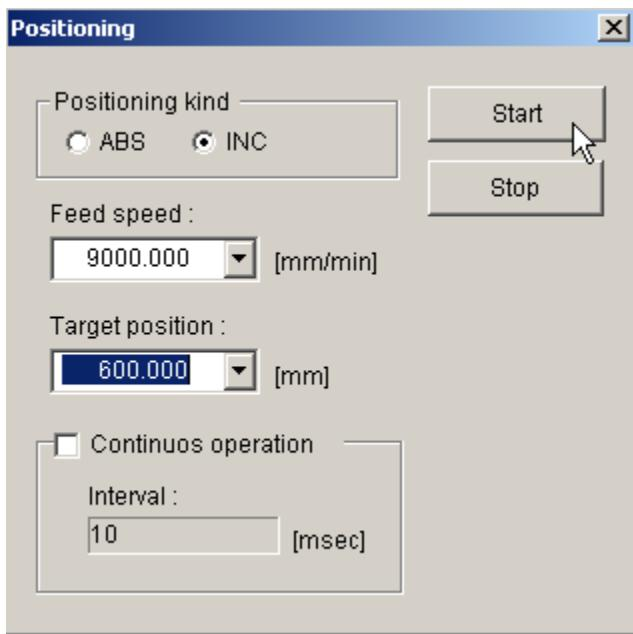
In the Positioning screen, select radio button INC. Set the value of 9000.00 in mm/minute (R.U. per minute). Set the target position of 600.000 mm. Press the start button. With current parameters of NSXXXDD.PRM, the motor should move close to 100 rev.
