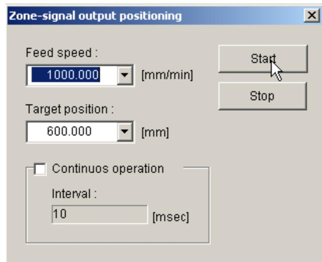
The Notch (zone signal) output mode allows two outputs CN4 (12), (10) to turn on and off at specified positions. NSXXXSTD.PRM sets the following parameters.
