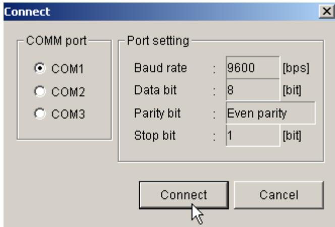
If the connection between your PC and NS300 /NS500 is not established, then close the set up tool software and try a different COM port. At the same time make sure a serial cable YS-16 is connected to the CN11 connector with correct orientation.
