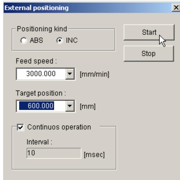
Enter the speed of 3000 mm/min in the Feed speed window. Enter the target position of 600.000 mm in the target position window. This speed and target position is the initial speed and position, before the EXTP (CN1-44) is turned ON.
