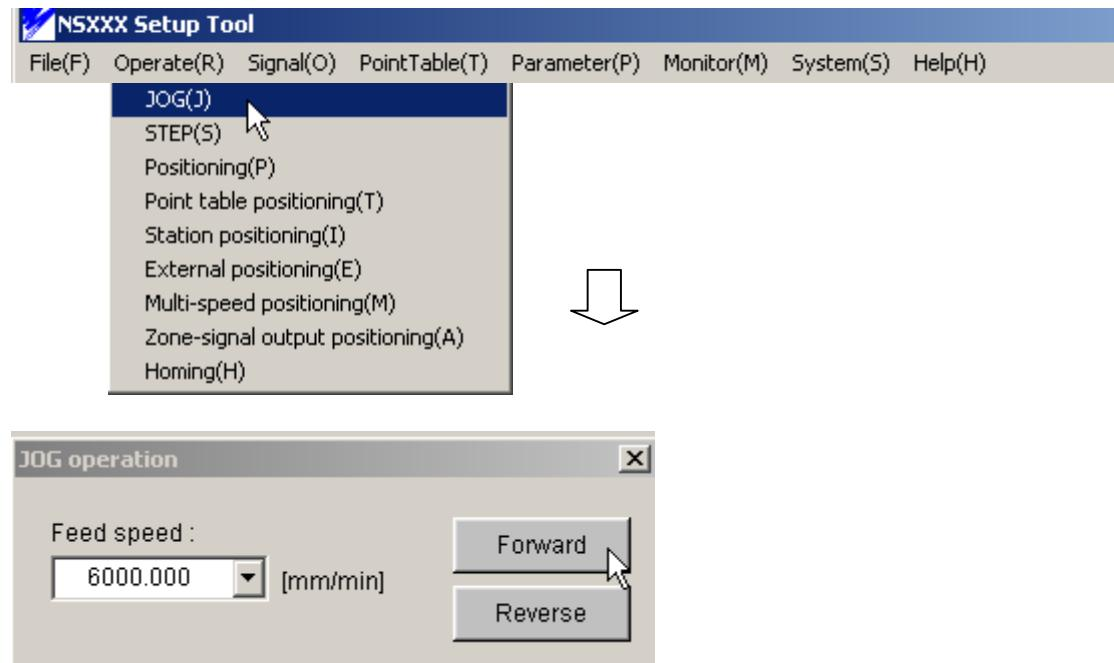
Select a speed in Reference units per minute (6000.00 mm/min) and select Forward or Reverse. The servomotor should rotate at the speed set in the Feed speed box. As per the calculation above, the motor will run at a speed of 1000 rpm.
