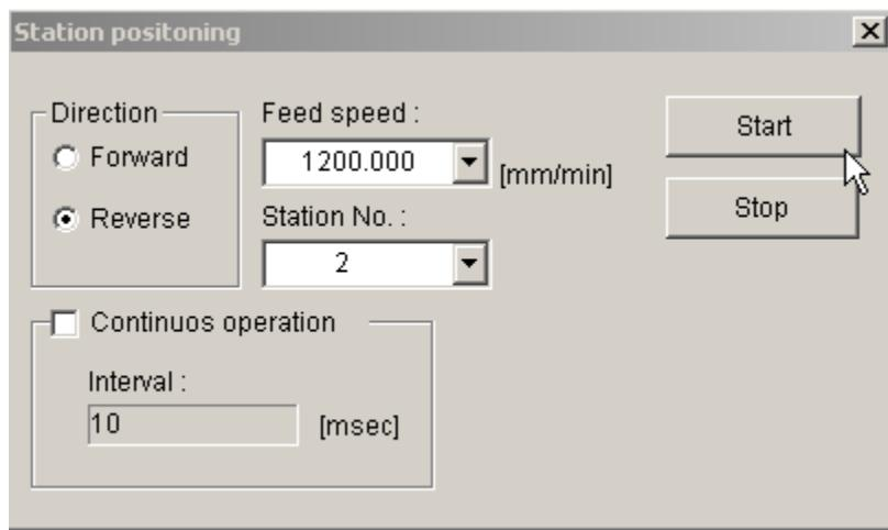
The NS300/NS500 has a station-positioning mode for rotary tables. The number of R.U per one machine rotation is defined in parameter Pn813. The number of station's used
