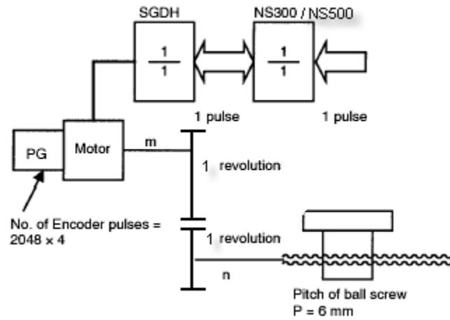
Let us set the Electronics gear ratio Pn810, Pn811, the maximum feed speed Pn843, feed speed for positioning and constant feed speed (for jogging) and ( Pn 821,Pn831 and Pn831) are set to the **default 24000 [R.U./min]**.
